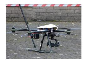
Figure 34. UAV used for photogrammetry measurements (Brussels case study)
