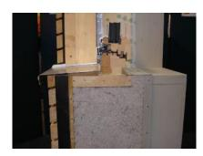
Figure 62. Prototype illustrating the blown adaptation layer (<u>Pettenbach</u>, AT)
