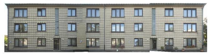
Figure 31. 'Pseudo-orthophoto' obtained from the lens distortion treatment and the perspective rectification (Brussels case study)
