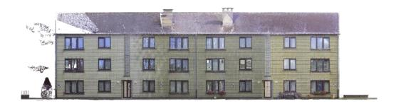
Figure 28. An 'Orthophoto', which is the equivalent of a textured elevation, can be created from TLS data (Brussels case study)
