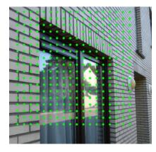
Figure 26. Principle of TLS measurement. The edges of an object are not directly detectable (Brussels case study)
