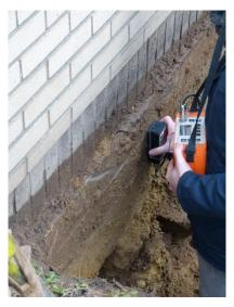
Figure 42. Characterization of the foundation system with a pachometer
