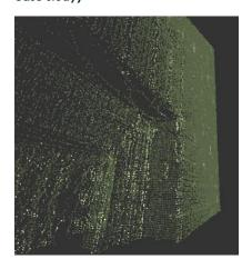
Figure 27. Raw data from TLS: The edges of an object are not directly detectable but the high resolution allows to find points really near to them (Brussels case study)
