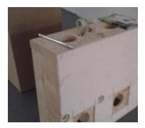
Figure 117. Through-hole mounting method presenting a higher risk of thermal bridges (Berlin, DE)
